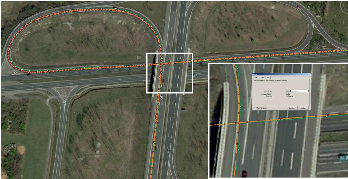
Figure 7.11: Map-section on a highway. Plotted are the fixed tight-coupled solution (orange) and the reference-solution (green)
