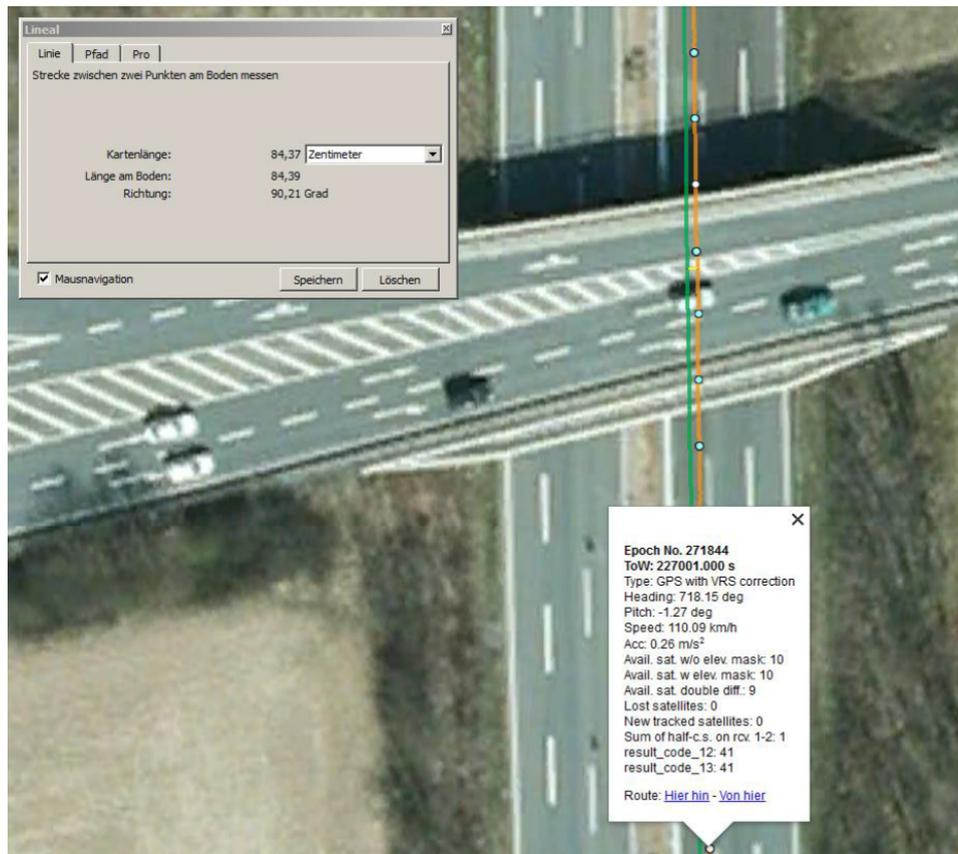
Figure 7.12: Map-section on a highway below a bridge. Plotted are the fixed tight-coupled solution (orange) and the reference-solution (green)
