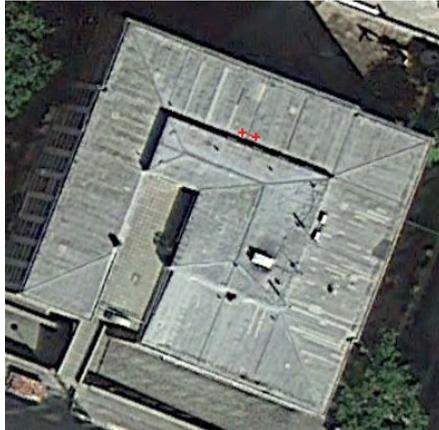
**Figure 3.1:** Static short-baseline test set-up. Crosses mark the positions of the test receivers
