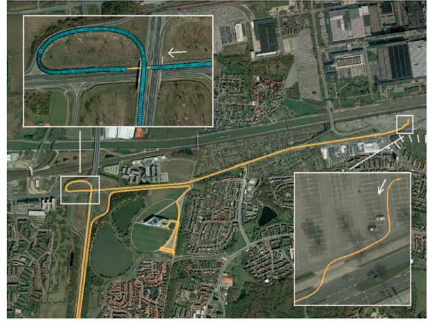
Fig. 5. Northern part of vehicle's track during test drive as determined by proposed PPP with tight coupling of two low-cost GNSS receivers, a gyroscope, and an accelerometer. Enlarged sections show start and passing below a bridge. Each blue point refers to GPS-based state update.
